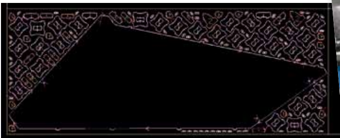
An example of how we can minimise material waste by nesting items that use the same material.
